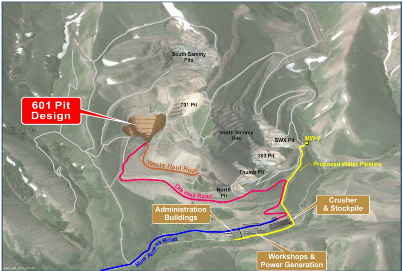
Figure 1: Oblique view of proposed site layout for mining of the current 601 pit design.
